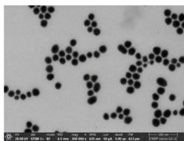
Figure 4. Imagini STEM: (A) Da (AuNPs-PEG-NH-PEG-epoxy-PEI-GA) (Schema 1.B.); (B) Db (AuNPs-PEG-PEI-GA) (Schema 1.A.).
